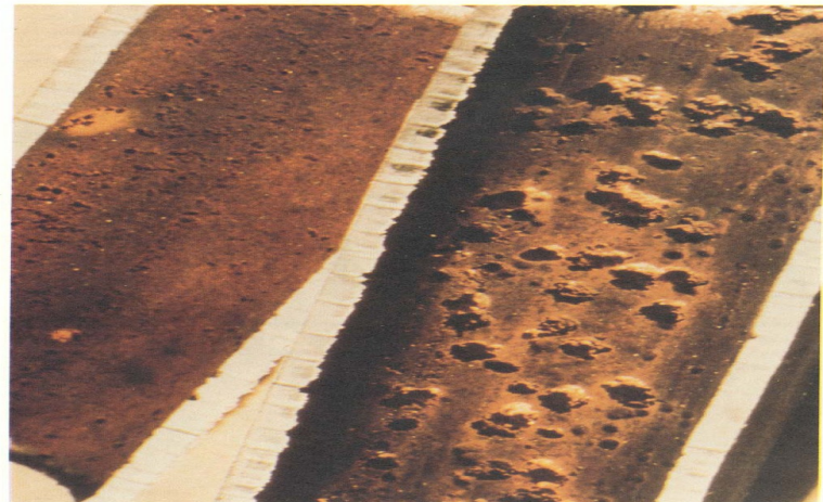
Figure 7-10. Pitting Damage from Localized Corrosion. Localized pitting results when electrochemical galvanic cells are established on the tube surface due to a difference in oxygen concentration in the boiler water and within a surface deposit or a crevice. Metal loss will occur at sites where the oxygen concentration is lower than that of the boiler since these locations become the anodes of the cell. Source: Beta Laboratories, Inc.
